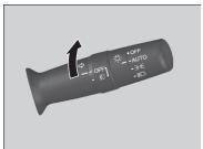
**To turn the front fog lights on:** Rotate the switch to the ฆ . The ฆ indicator comes on.
