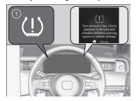
Low Tyre Pressure/Deflation Warning System Indicator This will cause the low tyre pressure/deflation warning system indicator to come on and a message to appear on the gauge.
