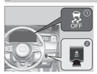
1 VSA OFF Indicator 2 2 (VSA OFF) Button This button is on the driver side control panel. To partially disable VSA functionality/features, press and hold it until you hear a beep.
