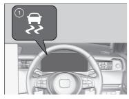
motor does not respond to the accelerator. You may also notice some noise from the hydraulic brake system. You will also see the indicator blink.
