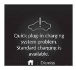
■ Reasons for the warning to appear Appears when there is a problem with the quick plug-in charging system or the charging station outlet.
