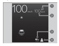
When ACC with Low Speed Follow starts operating, the vehicle icon, interval bars, and set speed appear on the gauge.
