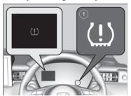
This will cause the low tyre pressure/deflation warning system indicator to come on and a message to appear on the gauge.
