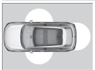
When you carry the keyless remote, you can lock/unlock the doors and tailgate.
