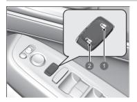
Press the master door lock switch in as shown to lock or unlock all the doors and tailgate.
