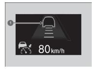
1 A vehicle icon with line contour appears on the gauge.
