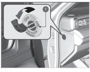
Passenger Front Airbag ON/ OFF Switch
