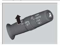
When the low beam headlights are on, turn the fog light switch on to use the fog lights.
