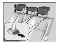
A passenger sitting in the outer or centre\* back seating position should adjust the height of their head restraint to an appropriate position before the vehicle begins moving.
