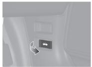
Locate the bonnet latch lever, push it to the side, and then raise the bonnet. Once you have raised the bonnet slightly, you can release the lever.
