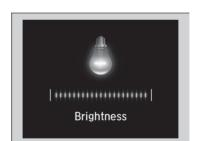
When the power mode is in ON, you can use the + or - button to adjust instrument panel brightness.
