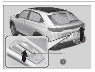
When all the doors are unlocked, the tailgate is unlocked. Press the tailgate outer handle and lift open the tailgate.
