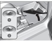
The driver's and front passenger's\* floor mats hook over the floor anchors, which keep the mats from sliding forward. When reinstalling the mats after cleaning, position them properly.
