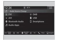
Select **Audio Source** on the header area, then select an icon on the source list to switch the audio source.
