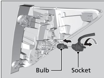
3. Turn the socket anticlockwise and remove it. Remove the old bulb.
