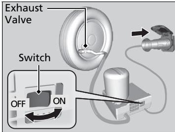
8. Turn the air compressor switch on to inflate the tyre.
