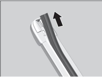
**3.** Slide the wiper blade out of the holder by pulling the tabbed end out.
