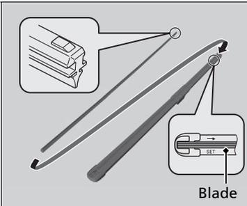
**4.** Slide the new wiper blade onto the holder from the bottom end.
