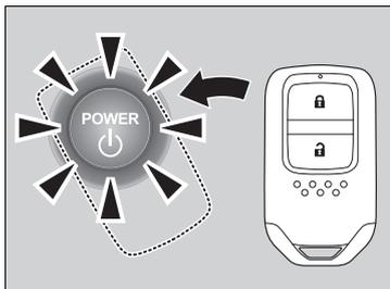
1. Touch the centre of the **POWER** button with the **H** logo on the keyless remote while the **POWER** button is flashing. The buttons on the keyless remote should be facing you.
