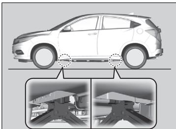
7. Place the jack under the jacking point closest to the tyre to be changed.
