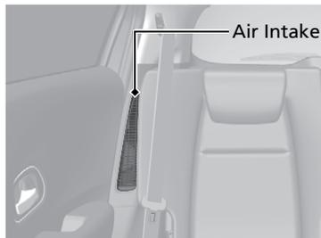
If the air intake is obstructed during vehicle operation, the High Voltage battery can become too hot. To protect the battery, the system may limit the battery's output and cause the power system and 12-volt battery charging system indicators to come on.
