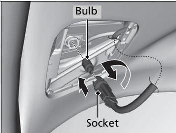
2. Turn the socket anticlockwise and remove it.
