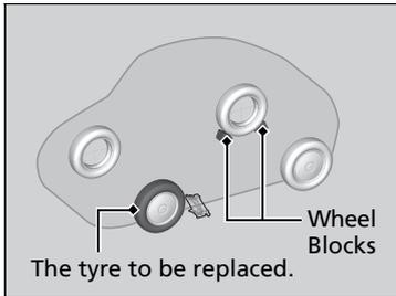
1. Place a wheel block or rock in front and rear of the wheel diagonal to the flat tyre.
