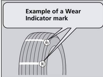
The groove where the wear indicator is located is about 1.6 mm shallower than elsewhere on the tyre. If the tread has worn so that the indicator is exposed, replace the tyre.
