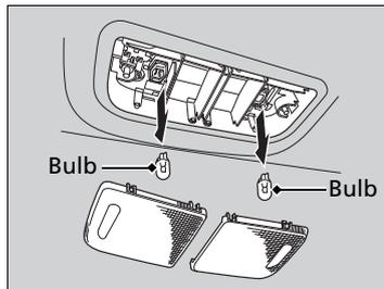
2. Remove the old bulb and insert a new bulb.
