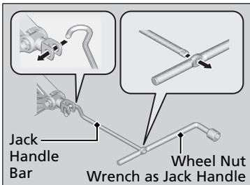
9. Raise the vehicle, using the jack handle bar and the jack handle, until the tyre is off the ground.
