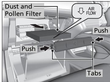
5. Push in the tabs on the corners of the filter case cover, and remove it.
