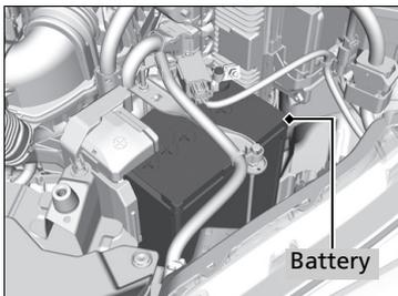
The condition of the battery is monitored by a sensor located on the negative terminal of the battery. If there is a problem with this sensor, the multi-information display will display a warning message. If this happens, have your vehicle inspected by a dealer.
