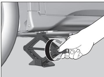
8. Turn the end bracket clockwise as shown in the image until the top of the jack contacts the jacking point.
