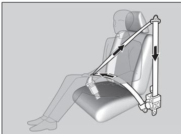
The tensioners automatically tighten the front seat belts during a moderate-to-severe frontal collision, sometimes even if the collision is not severe enough to inflate the front airbags.
