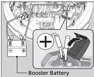
1. Open the fuse box cover on the positive  $\oplus$  terminal.
