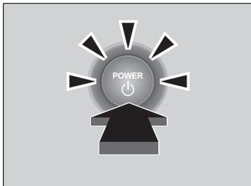
2. Depress the brake pedal and press the **POWER** button within 10 seconds after the beeper sounds and the **POWER** button stays on.
