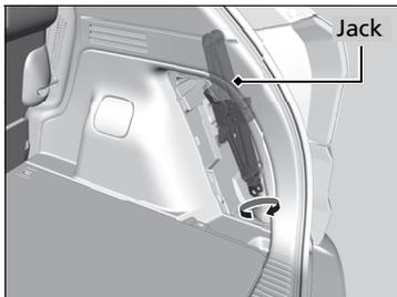
6. Turn the jack's end bracket clockwise to loosen it, then take the jack out.
