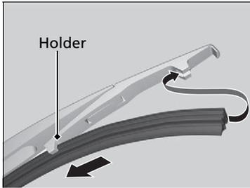
**5.** Slide the new wiper blade onto the holder.
