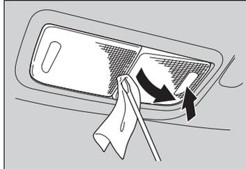
1. Pry on the edge of the cover using a flat-tip screwdriver to remove the cover.
