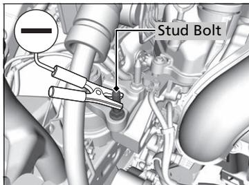
5. Connect the other end of the second jumper cable to the stud bolt as shown. Do not connect this jumper cable to any other part.
