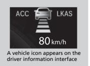
When a vehicle whose speed is slower than your set speed comes in or cuts in front of you and is detected by the radar and the camera, your vehicle starts to slow down.
