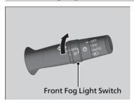
■ To turn the front fog lights on Rotate the switch to \$○. The \$○ indicator comes on.
