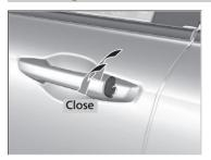
**To close:** Lock the driver's door with the key. Within 10 seconds of returning the key to the central position, turn the key in the lock direction and hold it there.
