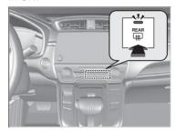
The rear demister automatically switches off after 10-30 minutes depending on the outside temperature. However, if the outside temperature is 0°C or below, it does not automatically switch off.
