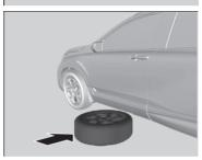
**8.** Place the spare tyre under the vehicle body (wheel side up) near the tyre that needs to be replaced.
