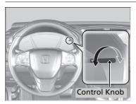
When the brightness of the meter will be reduced, you can use the brightness control knob to adjust instrument panel brightness. **Brighten:** Turn the knob to the right. **Dim:** Turn the knob to the left
