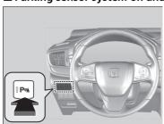
With the power mode in ON, press the parking sensor system button to turn on or off the system. The indicator in the button comes on when the system is on.
