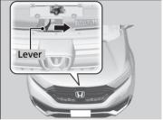
3. Push the bonnet latch lever (located under the front edge of the bonnet to the centre) to the side and raise the bonnet. Once you have raised the bonnet slightly, you can release the lever.
