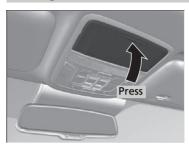
To open the sunglasses holder, press and release the indent. To close, press it again until it latches.
