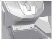
Connect a device to the input jack using a 3.5 mm stereo miniplug.
