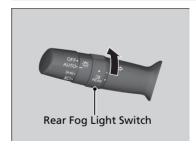
■ To turn the rear fog light on Rotate the switch to ()‡. The ()‡ indicator comes on.
