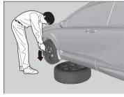
**9.** Loosen each wheel nut about one turn using the wheel nut wrench.
